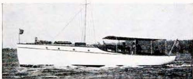
40 ft. Elco Cruiser. Sleeps Seven. 20 horse power Standard Gasoline Engine. Designed for ocean cruising.
