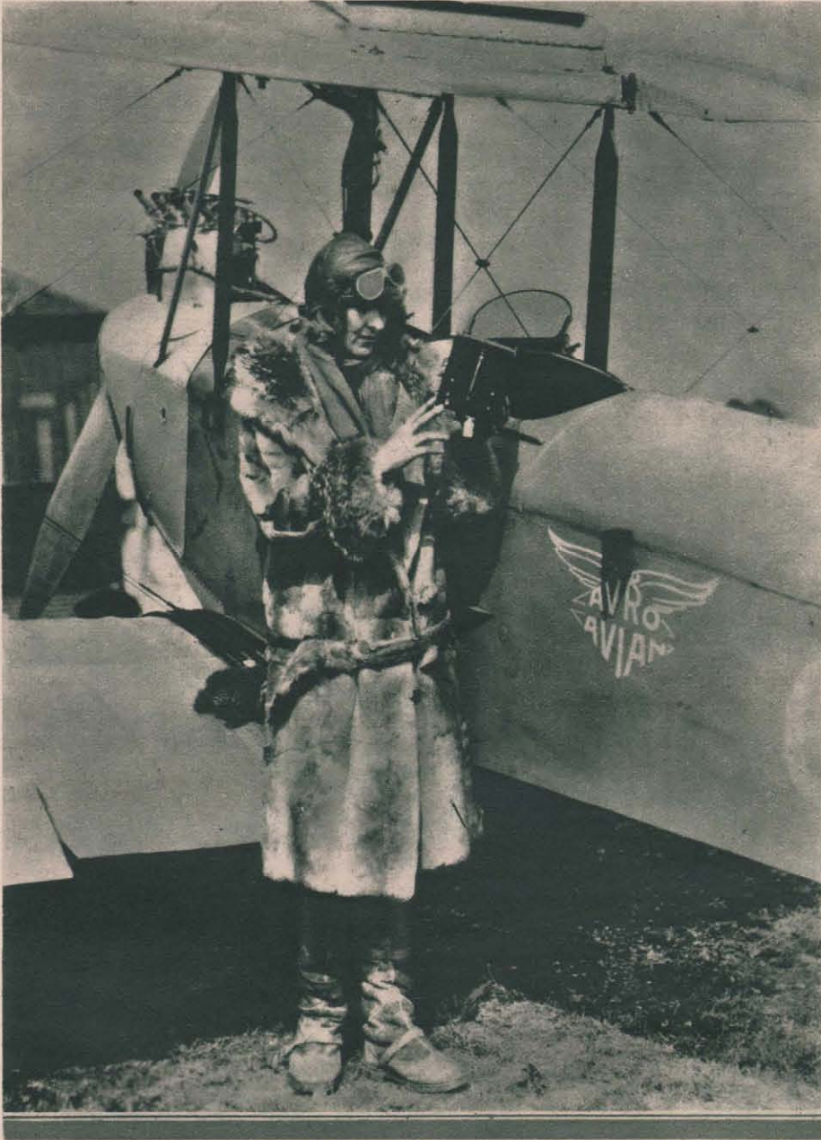
Examining the barograph before going up for her first attempt at the altitude record in May, 1927. The barograph is an altitude recorder
