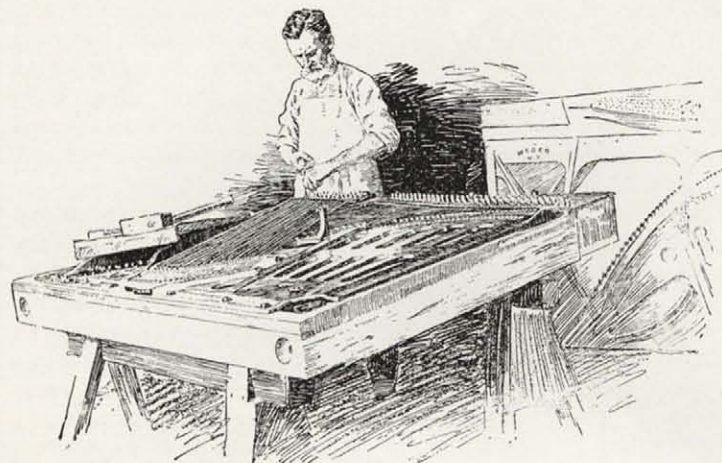
PUTTING STRINGS IN PLACE ON UPRIGHT PIANO.
