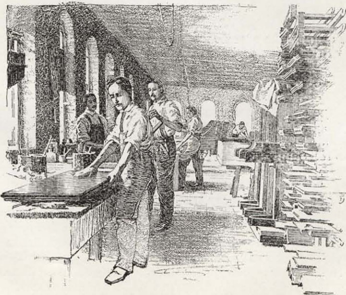
POLISHING TOPS, COVERS, AND CASINGS.
