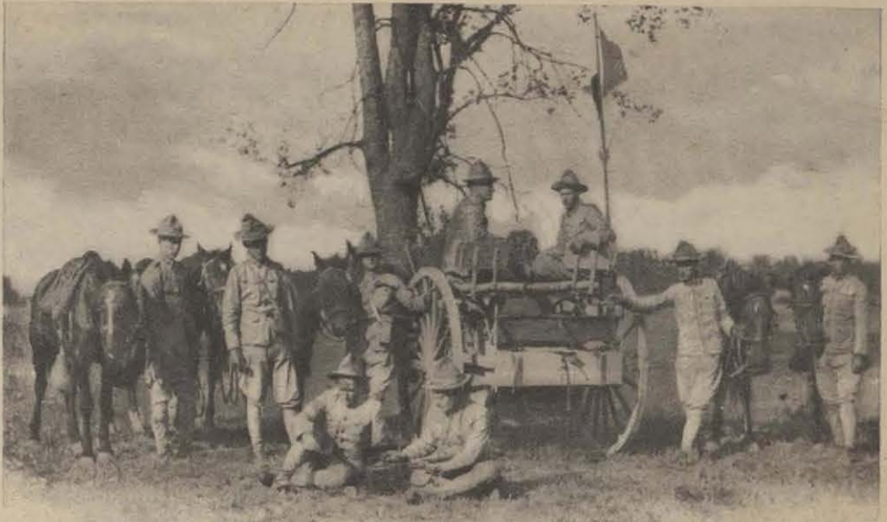
A FIELD TELEGRAPH-STATION OF THE UNITED STATES ARMY SIGNAL CORPS—THE MEN ON THE GROUND HAVE ESTABLISHED TELEPHONIC COMMUNICATION WITH ANOTHER STATION
