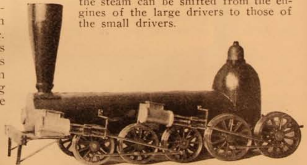
MODEL OF ENGINE PATENTED BY G. A. NICOLLS IN 1848 WITH SMALL AND LARGE DRIVERS SO IT COULD BE OPERATED INDEPENDENTLY FOR FREIGHT AND PASSENGER SERVICE.
