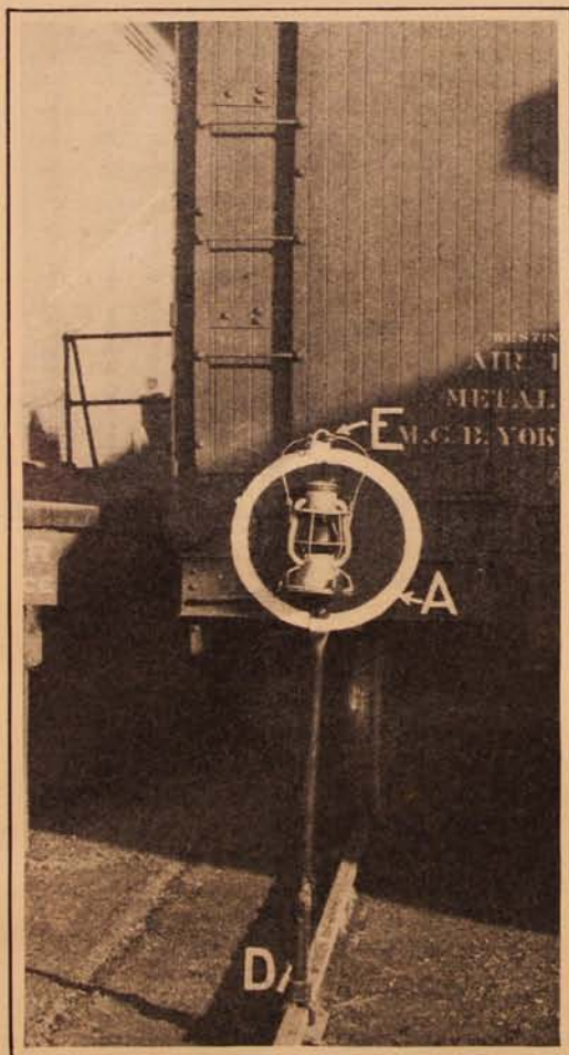
TRACK TARGET FOR NIGHT AND DAY SERVICE. A.—TRACK DISK PAINTED RED WITH OUTER RING OF WHITE. D.—CLAMP FOR SECURING TARGET TO RAIL. E.—PADLOCK ON LANTERN TO PREVENT REMOVAL.
